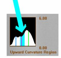
For a joint with a large toe region, set the start upward curvature to 35 to 45 and set the end upward curvature to 65 to 75. The goal is the place the search region in blue around the point where the solder flows up to create the toe.
