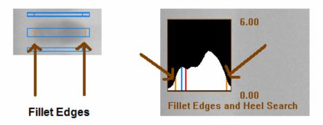
If the fillet edge graphics are near the edge of the Fillet edges and Heel search graphics window, then the pad length needs to be increased to allow the algorithm to find the edges correctly. Adjust the Pad Profile Length if necessary.
